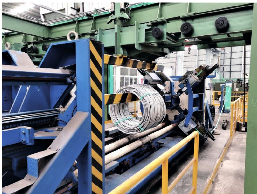
REPCH3-4600R-PS 25/32 horizontal coil compactor with PET strap, in a mill.
