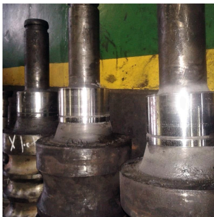
Shafts with laser-repaired surfaces.
