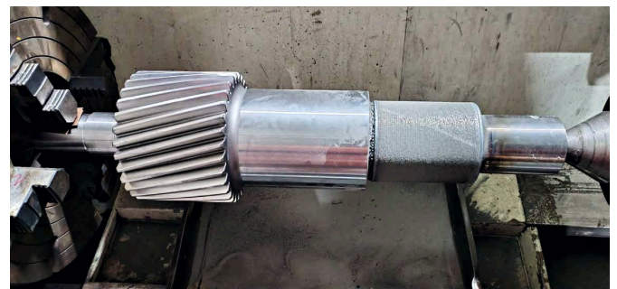
Laser-clad journal on a gear shaft.
