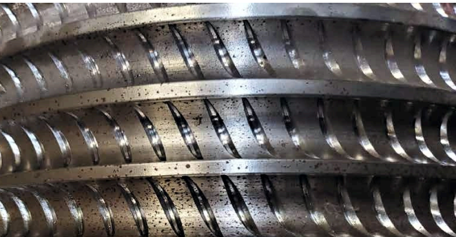
Rib grooves milled into a roll.
