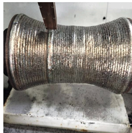
Guide roller after laser cladding.
