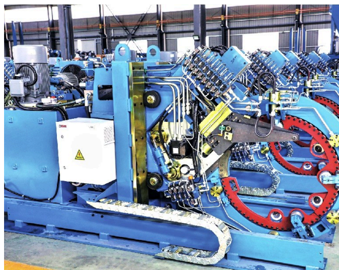
REBM1-800D-W7-A master bundle binding machine.
